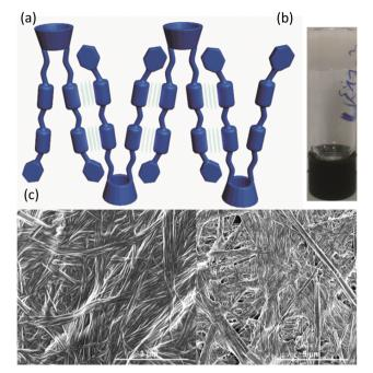
(a) Schematic of the proposed self-assembly of 1 to produce a gel fibre (b) vial inversion test of the 1,2-dibromoethane gel of 1 (2% w/v) (c) SEM images of the xerogel
