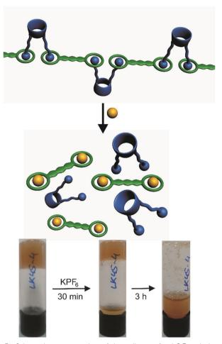
Fig. 5 Schematic representation of the collapse of gel 2.3 and photographs of the gel samples upon addition of upon addition of KPF<sub>6</sub> in acetonitrile solution.
