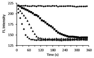
Fig. 5 Real-time assay of PPi (80  $\mu$ M) hydrolysis catalysed by different amounts of pyrophosphatase ( $\bullet$  = 0 units,  $\blacksquare$  = 0.5 units,  $\blacktriangle$  = 1.0 units,  $\bullet$  = 2.0 units) in the presence of  $\mathbf{3} \cdot \mathbf{Zn_2}$  (15  $\mu$ M) in Tris buffer (10 mM, 10 mM MqCl<sub>2</sub>, pH 7.5) at 30 °C,  $\lambda_{ex}$  = 390 nm, slits = 5 nm & 5 nm.
