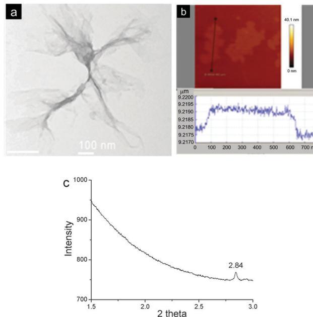
**Fig. 2** (a) TEM image of the SOF fabricated from **1** (0.0125 mM) and CB[8] (0.0188 mM), (b) tapping-mode AFM image and section analysis of the SOF fabricated from **1** (0.0125 mM) and CB[8] (0.0188 mM), and (c) synchrotron SAXS profiles of the SOF obtained by evaporating its solution. The SOF was prepared by dissolving a mixture of **1** and CB[8] (2 : 3) in water–methanol (17 : 3, V/V) and standing overnight without disturbance at room temperature.
