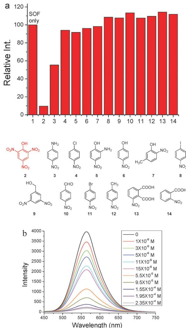
Fig. 4 (a) Changes in the fluorescence intensity of the 2D SOF upon the addition of different nitroaromatics, and (b) fluorescence spectra of the 2D SOF in the presence of different amounts of PA in water. The concentration of **1** in the SOF was  $2.0 \times 10^{-7}$  M.
