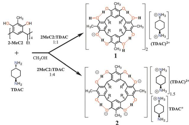
Fig. 1 Synthesis of mono- (**1**) and tetra-anions (**2**) from 2-methyl-resorcinarene (**2-MeC2**) and *trans*-1,4-diaminocyclohexane (**TDAC**). Nomenclature: **TDAC** = *trans*-1,4-diaminocyclohexane; **(TDAC)<sup>+</sup>** = *trans*-1-ammonium-4-aminocyclohexane; **(TDAC)<sup>2+</sup>** = *trans*-1,4-diammonium-cyclohexane.
