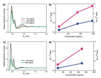
Fig. 3 (a) Strength of cation-anion affinity in IL-I. (b) The numbers of counterions in 1st (blue line) and 2nd (red line) shell of IL-I. (c) Strength of cation-anion affinity in IL-Cl. (d) The numbers of counterions in 1st (blue line) and 2nd (red line) shell of IL-Cl. Strength of cation-anion affinity is expressed in terms of cation-anion radial distribution function, at rising concentration of IL
