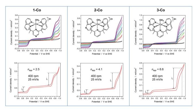
Fig. 6 RDEV of the series of cobalt catalysts. *Panels*: axial isomer **1-Co**,  $[(ax-PY4PZMe_2)Co(OH_2)]^{2+}$ ; equatorial isomer **2-Co**,  $[(eq-PY4PZMe_2)Co(OH_2)]^{2+}$ ; and catalyst **3-Co**,  $[(PY3PZ2Me_2)Co(OH_2)]^{2+}$ . *Top*: rotation rates of 100-3600 rpm; *bottom*: apparent  $n_{app}$  based on  $1e^{-}$  Co(III/III) couple at 400 rpm. *Conditions*: 0.3 mM catalyst, 0.1 M pH 7 KPBS, 0.1 M KNO<sub>3</sub>, 25 mV s<sup>-1</sup> scan rate, glassy carbon electrode (3 mm dia).
