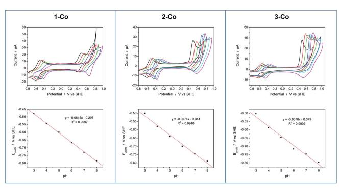
Fig. 5 Cyclic voltammograms as a function of pH and plots of the first reductive peak potential ( $E_{p,c(1)}$ ) vs. pH for 1-Co, 2-Co, and 3-Co. Conditions: 0.9 mM catalyst, 0.03 M buffer, 0.1 M KNO<sub>3</sub>, 100 mV s<sup>-1</sup> scan rate, glassy carbon electrode (3 mm dia). Note: CV at pH 7 is omitted for clarity in series of CVs for 1-Co. Legend: pH 3 (black), pH 4 (red), pH 5 (green), pH 6 (blue), pH 7 (cyan), pH 8 (magenta).
