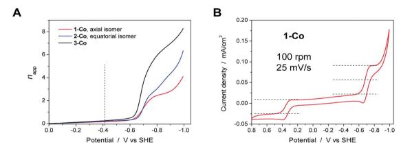
Fig. 7 A. Comparison of  $n_{\rm app}$  vs. applied potential for catalysts **1-Co** (red), **2-Co** (blue), and **3-Co** (black) based on steady-state voltammograms in Fig. 6 (bottom). The vertical dashed line denotes the thermodynamic potential for water reduction at pH 7. B. Steady-state voltammogram of catalyst **1-Co** at 100 rpm, 25 mV s<sup>-1</sup>.
