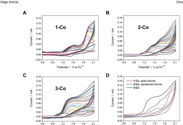
Fig. 3 Cyclic voltammetry of catalysts (1 mM) in acetonitrile with various concentrations of chloroacetic acid (up to 20 equivalents, 20 mM). A, B, and C. Catalysts **1-Co**, **2-Co**, and **3-Co**, respectively. The CV in black in these three graphs is the indicated catalyst in the absence of acid. D. Comparison of CVs for each catalyst, **1-Co** (red), **2-Co** (blue), and **3-Co** (black), with 20 eq. of chloroacetic acid. Scan rate =  $100 \text{ mV s}^{-1}$ ; 3 mm dia. glassy carbon.
