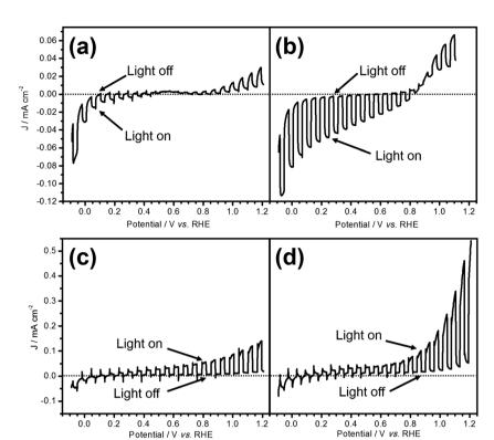
Fig. 1 Potential—current curves of (a) LTC/Au, (b) Pt/LTC/Au, (c) LTC/Ti, and (d) CoPi/LTC/Ti electrodes under visible light ( $\lambda$  > 420 nm) irradiation. The reference and counter electrodes used were an Ag/AgCl electrode and Pt wire, respectively. The potential was scanned in the positive direction.
