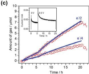
Fig. 2 Evolution of hydrogen/oxygen from the two-electrode system under visible light ( $\lambda$  > 420 nm) irradiation. (a) Pt/LTC/Au (3.5 cm²) – Pt wire under a bias of -0.9 V, (b) CoPi/LTC/Ti (4.3 cm²) – Pt wire under a bias of 0.8 V and (c) CoPi/LTC/Ti (4.5 cm²) – Pt/LTC/Au (2 cm²) under a bias of 0 and 0.5 V. The inset shows current–time curves recorded during the respective measurements.
