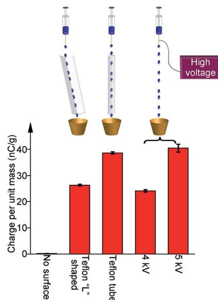
Fig. 4 An electrical potential of ~4–5 kV from a power supply was required to generate the amount of charge in a water droplet similar to that generated by contacting the droplet with either a L-shaped channel or a tube. When water droplets were not in contact with any solid surface, they did not contain any charge.
