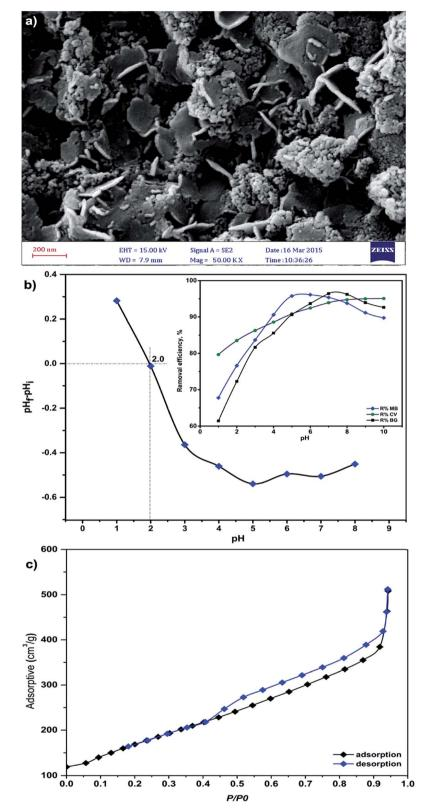
Fig. 4 (a) FESEM image of the prepared MnO<sub>2</sub>-NP-AC, (b) pHzpc of MnO<sub>2</sub>-NP-AC (pH $_i$  = initial pH and pH $_f$  = final pH) and (c) nitrogen adsorption–desorption isotherms.
