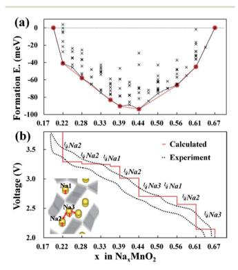
Fig. 6 (a) Formation energies of seven stable intermediate phases during  $Na_xMnO_2$  cycling calculated from 156 different sodium configurations, and (b) experimental and calculated voltage profiles for  $Na_xMnO_2$  with respect to the minimum energy path of formation energies. Reproduced with permission<sup>35</sup> © 2012, ACS Publications.
