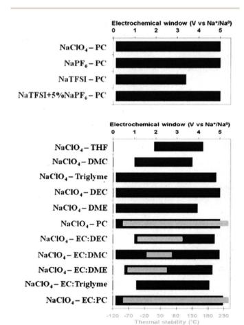
Fig. 15 Electrochemical potential window stability of various salts with PC and NaClO $_4$  in various solvents. Reproduced with permission $^{150}$  © 2012, RSC Publishing.
