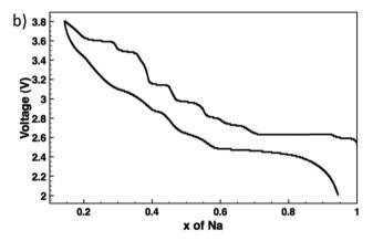
Fig. 4 Voltage profiles: (a)  $Na_xMnO_2$  cycled at C/10 with the cycle numbers indicated, and (b)  $Na_xMnO_2$  de/sodiation as measured by potentiostatic intermittent titration. Reproduced with permission<sup>36</sup> © 2012, The Electrochemical Society.
