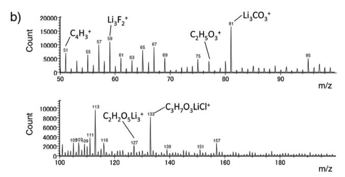
Fig. 21 TOF-SIMS positive ion spectra for the hard-carbon electrodes after the first galvanostatic cycle in (a) sodium and (b) lithium cells. Reproduced with permission<sup>128</sup> © 2011, WILEY-VCH Verlag GmbH & Co.
