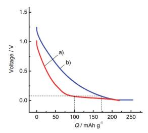
Fig. 19 Chronopotentiograms of the second reduction for hardcarbon electrodes in (a) 1 mol dm<sup>-3</sup> NaClO<sub>4</sub> and (b) 1 mol dm<sup>-3</sup> LiClO<sub>4</sub> PC solution in Na and Li cells, respectively, at a rate of 25 mA  $g^{-1}$ . Reproduced with permission<sup>128</sup> © 2011, WILEY-VCH Verlag GmbH & Co.
