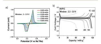
Fig. 10 (a) Cyclic voltammogram of Na $_3$ V $_2$ (PO $_4$ ) $_3$ , and (b) galvanostatic charge and discharge profiles for several C rates. Reproduced with permission $^{\rm g1}$  © 2013, WILEY-VCH Verlag GmbH & Co.
