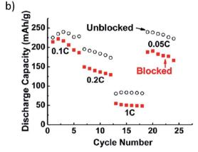
Fig. 13 (a) Na ions transport along and diffuse through the mesoporous wood fiber structure. Internal transport pathways are blocked by the conformal Al<sub>2</sub>O<sub>3</sub> coating, and (b) the rate performance of the Sn anode deposited on the carbon-coated mesoporous wood fibers. Reproduced with permission<sup>137</sup> © 2013, ACS Publications.
