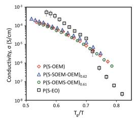
Fig. 5 Normalized ionic conductivity profiles for LiCF $_3$ SO $_3$ -doped P(S-OEM), P(S-SOEM-OEM) $_{0.62}$ , P(S-OEMS-OEM) $_{0.61}$ , and P(S-EO) at [EO]: [Li] = 15:1. The scaled conductivity profiles of POEM-based polymers fell onto a single master curve. The deviation between the P(S-EO) profile and the master curve likely was due to larger molar mass of PEO in P(S-EO) and PEO crystallization at lower temperatures.
