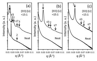
Fig. 2 APS-SAXS data for neat and LiCF $_3$ SO $_3$ -doped (a) P(S-OEM), (b) P(S-SOEM-OEM) $_{0.62}$ , and (c) P(S-OEMS-OEM) $_{0.61}$ . Data were shifted vertically for clarity.
