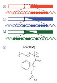
Fig. 1 Illustration of a (a) block polymer, (b) normal-tapered block polymer, and (c) inverse-tapered block polymer. (d) Molecular structure of P(S-OEM).
