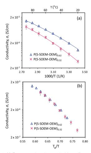
Fig. 7 (a) Temperature-dependent conductivity profiles and (b) normalized ionic conductivity profiles for LiCF<sub>3</sub>SO<sub>3</sub>-doped P(S-SOEM-OEM)<sub>0.62</sub> and LiCF<sub>3</sub>SO<sub>3</sub>-doped P(S-SOEM-OEM)<sub>0.32</sub> at [EO] : [Li] = 24:1. The reported values of ionic conductivity are averages from three samples with standard deviations indicated by error bars on the data points. The solid lines in (a) are VFT fits.
