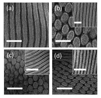
Fig. 3 TEM micrographs of (a) neat P(S-OEM), (b)  $LiCF_3SO_3$ -doped P(S-OEM), (c)  $LiCF_3SO_3$ -doped P(S-SOEM-OEM)<sub>0.62</sub>, and (d)  $LiCF_3SO_3$ -doped P(S-OEMS-OEM)<sub>0.61</sub>. The  $LiCF_3SO_3$ -doping ratio was [EO]: [Li] = 15:1. TEM samples were stained with  $RuO_4$  vapor to darken the POEM domains. Scale bars represent 50 nm.
