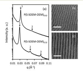
Fig. 6 (a) SAXS data for LiCF $_3$ SO $_3$ -doped P(S-SOEM-OEM) $_{0.62}$  and LiCF $_3$ SO $_3$ -doped P(S-SOEM-OEM) $_{0.32}$  at [EO] : [Li] = 24 : 1. Data were shifted vertically for clarity. TEM micrographs of (b) LiCF $_3$ SO $_3$ -doped P(S-SOEM-OEM) $_{0.62}$  and (c) LiCF $_3$ SO $_3$ -doped P(S-SOEM-OEM) $_{0.32}$ . TEM samples were stained with RuO $_4$  vapor to darken the POEM domains. Scale bars represent 50 nm.
