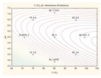
Fig. 10 Overlay contour plot for CCCD and SVM predictive model showing experimental points.
