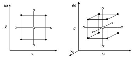
Fig. 2 Central composite designs for the optimization of: (a) two variables ( $\alpha = 1.41$ ) and (b) three variables ( $\alpha = 1.68$ ). ( $\bullet$ ) points of factorial design, ( $\bigcirc$ ) star points and ( $\square$ ) central point.
