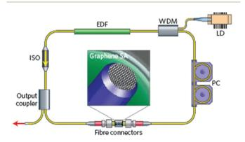
Fig. 76 Graphene fiber laser. 1353 WDM, wavelength division multiplexer; PC, polarization controller; EDF, erbium-doped fiber; ISO,
