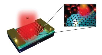
Fig. 80 Schematic of GQD hybrid phototransistor, in which a graphene flake is deposited onto Si/SiO<sub>2</sub> coated with PbS QDs. Incident photons create e-h pairs in the PbS QDs. [Adapted from ref. 1315].
