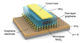
Fig. 66 MoS<sub>2</sub>/graphene heterostructure memory layout. 3d schematic view of the memory device based on 1L-MoS<sub>2</sub> semiconducting channel, SLG contacts and FLG floating gate. The FLG floating gate is separated from the channel by a thin tunnelling oxide and from the control gate by a thicker blocking oxide.
