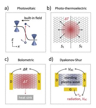
Fig. 78 Schematic representation of the four different photocurrent generation mechanisms, (a) photovoltaic, (b) photothermoelectric, (c) bolometric and (d) plasma wave-assisted (Dyakonov-Shur). Adapted from ref. 1434.
