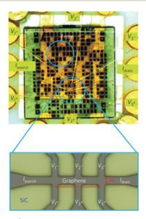
Fig. 33  $7 \times 7 \text{ mm}^2$  wafer of SiC with 20 Hall bar devices. The contact configuration for the smaller device is shown in the enlarged image.<sup>154</sup>
