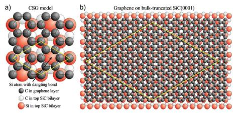
Fig. 46 (a) Top view of covalently bound stretched graphene (CSG) model on SiC(0001). (b) graphene on bulk-truncated SiC(0001) surface, Adapted from ref. 761.
