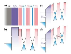
**Fig. 30** Graphene field-effect tunnelling transistor. (a) Schematic of the proposed devices. (b) The corresponding band structure with  $V_{\rm g}=0$ . (c) The same band structure for a finite  $V_{\rm g}$  and zero  $V_{\rm b}$ . (d) Both  $V_{\rm g}$  and  $V_{\rm b}$  are finite. The cones illustrate graphene's Dirac-like spectrum. Adapted from ref. 106.
