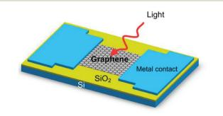
Fig. 77 Scheme of a MGM photodetector. Adapted from ref. 995.
