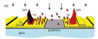
**Fig. 120** (a) Schematic plasmonic MZ interferometer. Adapted from ref. 2299. (b) Schematic plasmonic interferometer using grating coupling and an integrated graphene transducer.
