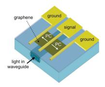
Fig. 79 Schematic of an integrated waveguide GPD
