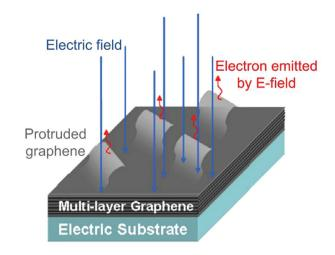
Fig. 70 Screen-printed graphene FE device.
