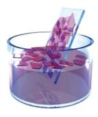
Fig. 52 Superstructure assembly by dispersions and inks. Dip casting is used to deposit successive layers of different 2d crystals to create an heterostructure.
