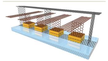
Fig. 60 Two cells graphene NOR gate flash memory. Graphene is used for conductive FET channels  $^{1140,1181}$  and bit line (black), control gates  $^{1180}$ and word lines (brown), and floating gates 1179 (white).
