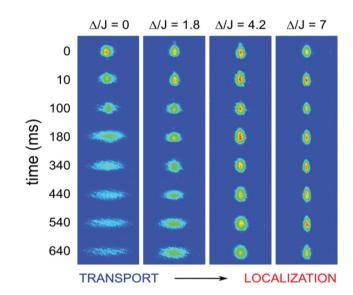
Fig. 23 Localization transition for 39 K ultracold atoms in a quasiperiodic bichromatic lattice: as  $\Delta$  is increased the atomic cloud becomes Anderson-localized. <sup>263</sup>
