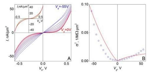
Fig. 69 (A) Tunnelling I-V s and their response to gate voltage (in 5 V steps) for a BN/SLG/(BN)<sub>4</sub>/SLG/BN device. <sup>106</sup> T = 300 K. (B) Changes in low-bias tunnelling (symbols) and the theory fit for 4 hBN layers (solid curve). Adapted from ref. 106.
