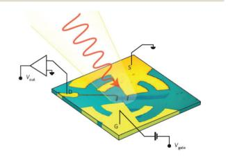
Fig. 81 Antenna-coupled GFET-terahertz detector. The terahertz radiation is focused by off-axis parabolic mirrors. Adapted from ref. 1445.
