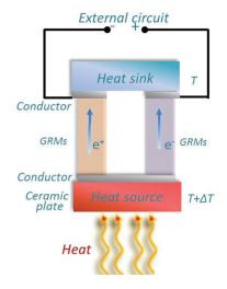
Fig. 105 Schematic illustration of power generation in a TE device based on  $Bi_2Te_3$  LMs or GNRs. A T gradient,  $\Delta T$ , causes charge carriers in the material to diffuse, resulting in current flow through the external circuit. Adapted from ref. 1841.
