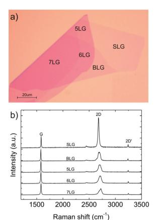
Fig. 40 (a) Optical micrograph of MC flake, with regions of different thickness. (b) Evolution of Raman spectra with N. 134 The spectra are normalized to have the same G peak intensity. 602
