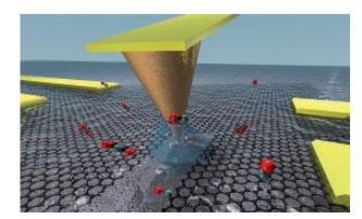
Fig. 24 AFM lithography of graphene. 306
