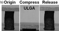
Fig. 111 (a) Photograph of an intermediate state of a sample on its way from ZnO to Aerographite.<sup>2155</sup> (b) Compressibility of GO based aerogel. ULGA is Ultralight and highly compressible Graphene Aerogels. Adapted from ref. 2157.
