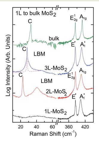
Fig. 27 Raman spectra of 1L-MoS $_2$ , 2L-MoS $_2$ , 3L-MoS $_2$ , and bulk MoS $_2$  measured at 532 nm. Adapted from ref. 204.
