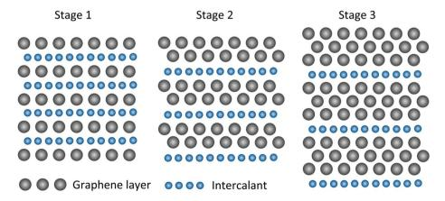
Fig. 45 Graphite intercalation compounds. In stage 1, SLG alternate with intercalant layers. In stage 2, stage 3, etc., 2, 3, etc. graphene layers separate two intercalant layers. Adapted from ref. 602.
