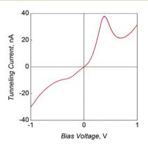
Fig. 29 /(V) characteristics of a SLG/4L-BN/SLG device. Adapted from ref. 106.
