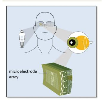
Fig. 115 Concept for an artificial retina based on a flexible GFET
