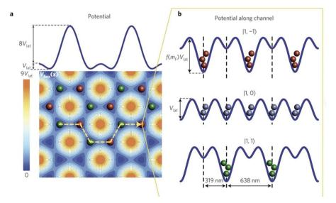
Fig. 21 (a) Lattice potential with alternating  $\pi^+$  (green spheres) and  $\pi^-$  (red spheres) polarization. The upper plot shows a cut through the 2d potential. (b) 1d potential along the channel of the orange dashed line in (a) for particles in different Zeeman states.<sup>284</sup>
