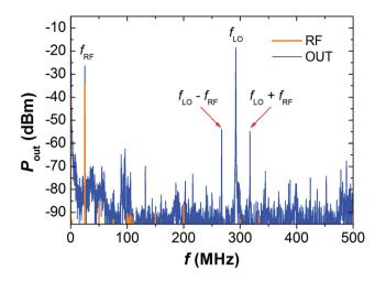
Fig. 65 Power spectrum of the output signal of a stand-alone graphene mixer at  $V_{\rm DD}$  = 2.5 V. The signal frequencies are  $f_{\rm LO}$  = 292 MHz and  $f_{\rm RF}$  = 25 MHz. Apart from the signals discussed in the text, the output signal also contains a frequency component at  $f_{\rm RF}$ , from the amplification of the RF signal by inverter 4 in Fig. 63.<sup>1102</sup>
