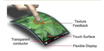
Fig. 95 Graphene-based electrotactile display. Adapted from ref. 1758.
