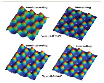
Fig. 20 Spatial distribution of electrons in AG (with one electron per pillar) calculated for two values of the potential well representing the pillar. The left and right panels show the results without and with e-e interactions.<sup>282</sup>
