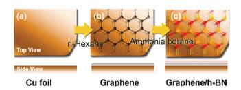
Fig. 51 Schematic of Graphene/BN stacked film. (a) The Cu foil is cleaned and prepared as the growth substrate. (b) High-quality and large-area graphene film is grown via CVD with n-hexane as a liquid carbon source at 950 °C. (c) The as-grown graphene is then loaded into another furnace for the growth of h-BN film on top. Adapted from ref. 1077.
