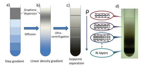
Fig. 41 Sorting of graphite flakes via isopycnic separation. Formation of (a) step gradient and (b) linear density gradient. (c)The flake-surfactant complexes move along the cuvette, dragged by the centrifugal force, until they reach their corresponding isopycnic points. The buoyant density of the flake-surfactant complexes increases with N. (d) Photograph of a cuvette containing sorted flakes. Adapted from ref. 602.
