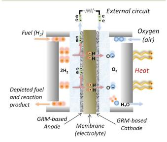
Fig. 100 Proton exchange membrane fuel cells.  $^{1911}$  Fuel (e.g.  $H_2$ ) channelled from one side of the fuel cell is split by catalyst (e.g. graphene electrode) into  $H^+$  ions and e-. Electrons generate a current in the external circuit and they combine with  $H^+$  and the oxidant  $(O_2)$  at the cathode forming water and heat. Adapted from ref. 1841.
