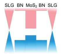
Fig. 31 SLG/h-BN/MoS<sub>2</sub>/h-BN/SLG structure: blue is the valence band and pink is the conduction band. Adapted from ref. 106.
