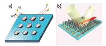
Fig. 119 (a) Illustration of graphene-passivated Ag nanoantennas fabricated in a square array. The graphene layer prevents the reaction of trace atmospheric hydrogen sulfide ( $H_2S$ ) and carbonyl sulfide (OCS) with the Ag surface. Adapted from ref. 2327. (b) Scheme of a square array of Au double-dots on a glass substrate covered by hydrogenated graphene. Adapted from ref. 2310.
