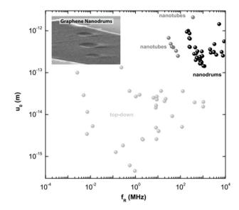
Fig. 86 Resonance frequency and zero-point motion measured for a large number of top-down and bottom-up CNT and graphene nanodrum resonators. Graphene nanodrums are capable of reaching GHz resonance frequencies (adapted from ref. 1674).
