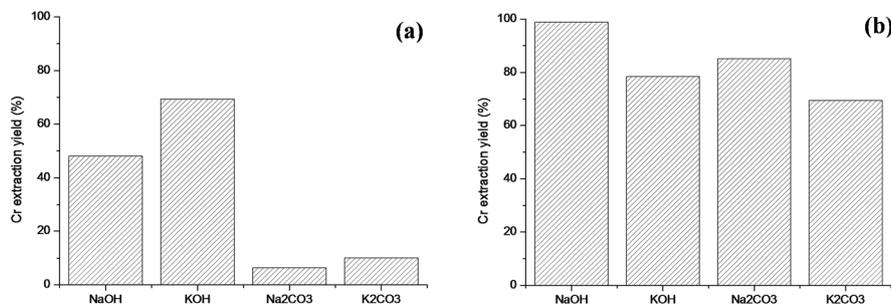
**Fig. 17** (a) Chromium extraction yields after roasting at 1000 °C for 2 hours in air and water leaching at 50 °C for 45 minutes with different alkali salts. (b) Chromium extraction yields after roasting at 1000 °C for 2 hours and water leaching at 50 °C for 45 minutes with different alkali salts under a richer oxygen atmosphere with intermittent stirring.
