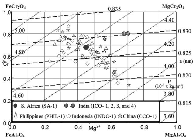
Fig. 2 The Deer's net superimposed on the reciprocal salt diagram for chromite ores. The dash lines (---) are for constant lattice parameter compositions ranging from  $0.815\text{ nm}$  to  $0.835\text{ nm}$ , whereas the constant density (dotted lines ...) of mineral changes from  $3.60\text{ g cm}^{-3}$  ( $= 3600\text{ kg m}^{-3}$ ) to  $5.00$  ( $= 5000\text{ kg m}^{-3}$ ) in the quaternary composition.<sup>19,20</sup>
