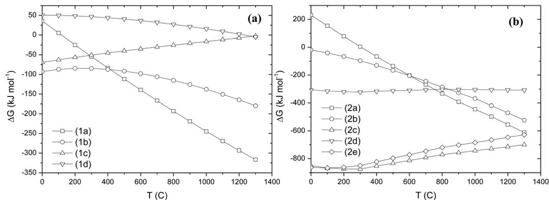
Fig. 8 (a) A plot of the standard Gibbs energy change ( $\Delta G^\circ$ ,  $\text{kJ mol}^{-1}$ ) per mol of mineral against temperature ( $T$   $^\circ\text{C}$ ) for: (a) thermal decomposition reactions (1a)–(1d), and (b) alkali roasting reactions (2a)–(2e).
