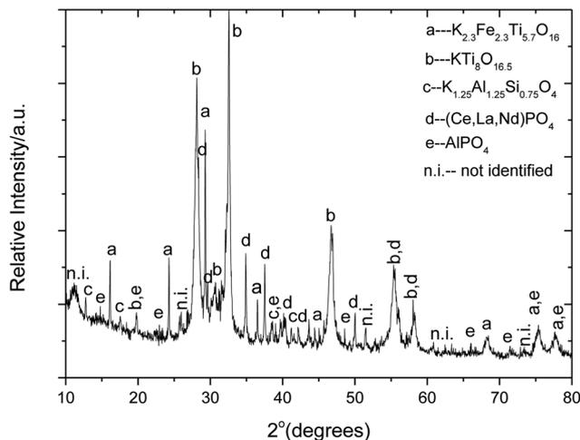
**Fig. 14** X-ray powder diffraction pattern of the reaction product formed as a result of chemical reaction between  $K_2CO_3$  and  $FeTiO_3$  at  $825\text{ }^\circ\text{C}$  for 4 hours in air. The main phases compare well with the ICDD references: 00-041-1100  $K_2O \cdot 8TiO_2$ , 00-040-0960  $K_{2.3}Fe_{2.3}Ti_{5.7}O_{16}$ , 00-032-0731  $K_{1.25}Al_{1.25}Si_{0.75}O_4$ , 00-046-1295  $(Ce, La, Nd)PO_4$  and 04-009-5769  $Al(PO_4)$ .
