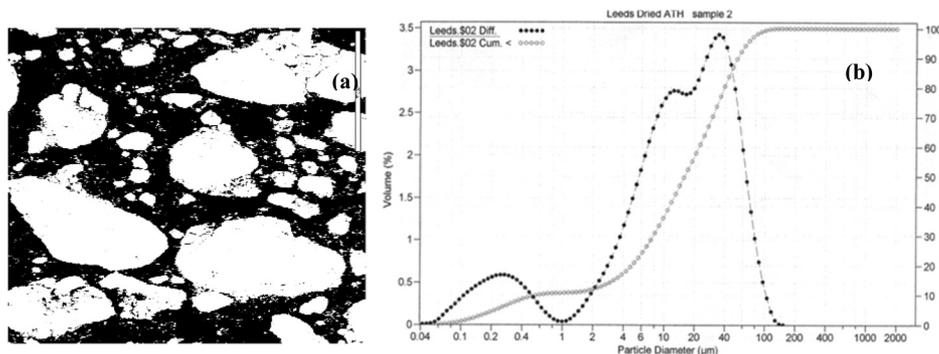
**Fig. 12** (a) Scanning electron micrograph of the alumina extracted (100  $\mu\text{m}$ ). (b) Cumulative distribution values with bimodal particle size distribution of calcined alumina.
