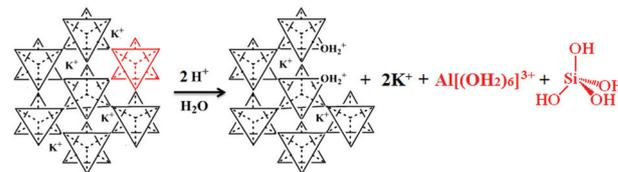
**Fig. 4** Schematic of the proton-promoted dissolution of K-bearing tecto-aluminosilicates, illustrating the dissolution of one cluster. The tetrahedra can contain Si or Al.
