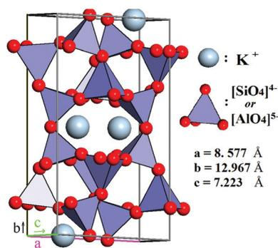
**Fig. 2** Idealized crystalline structure of microcline: the red spheres represent oxygen atoms; silicon and aluminum atoms are within the  $[SiO_4]^{4-}$  and  $[AlO_4]^{5-}$  tetrahedra, and the potassium charge-balancing cations are the blue spheres.
