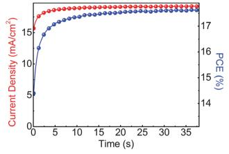
Fig. 3 Stabilized current density and power output measured close to the maximum power point (~0.92 V) for a photovoltaic device of glass/FTO/ TiO<sub>X</sub>/60-PCBM/CH<sub>3</sub>NH<sub>3</sub>Pbl<sub>3</sub>/spiro-MeOTAD/Au
