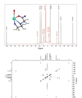
Fig. 3 Top:  $^1\text{H}$  NMR spectra (400 MHz, 298 K, D<sub>2</sub>O) of YbDTMA in the absence (black) and presence (red) of an excess of sodium fluoride, with assignments based on the labelled portion of the complex shown (using DyDTMA crystal structure  $^{12}$ ). Bottom: EXSY spectrum of YbDTMA with fluoride at 298 K with a mixing time of 1 ms at 500 MHz.
