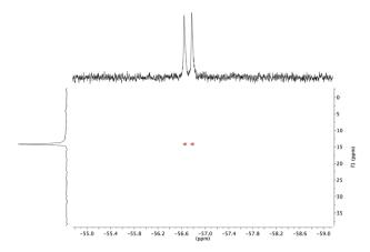
Fig. 2  $^{19}$ F detected  $^{89}$ Y $^{-19}$ F HMQC for a D<sub>2</sub>O solution of YDTMA and excess sodium fluoride with <sup>19</sup>F on the horizontal axis and <sup>89</sup>Y on the vertical axis. The coupling in the vertical dimension is refocused during the evolution delay.
