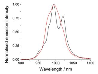
Fig. 1 Change in form of emission spectra with fluoride. Top: EuDTMA in D<sub>2</sub>O (black) and with excess sodium fluoride (red),  $\lambda_{\rm ex}$  = 394 nm, exit slit = 1 nm; inset shows the change in structure of the  $\Delta J$  = 1 band measured with 0.2 nm exit slit. Bottom: YbDTMA in D<sub>2</sub>O (black) and with added fluoride (red),  $\lambda_{\rm ex}$  = 265 nm, exit slit = 5 nm.
