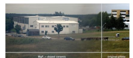
Fig. 17 Picture taken wherein the left side of the camera lens (2/3 of the image) is covered by the "new transparent ceramic" disc whereas the right side shows the original photo.
