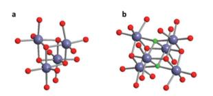
Fig. 10 Illustration of the molecular structures of magnesium methoxide (a) and the  $Mg_6F_2(OCH_3)_{10}(CH_3OH)_{12}$  dicubane (b).
