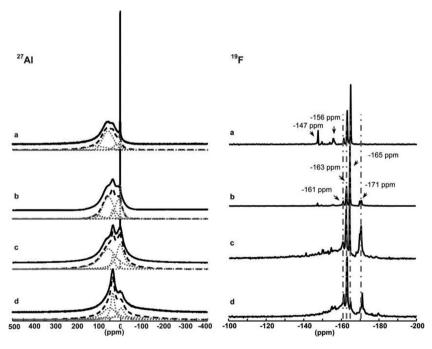
Fig. 4  $^{27}$ Al NMR and  $^{19}$ F NMR spectra of different sols and wet gels recorded at  $B_0 = 9.4$  T. Increasing fluorine content from a-d with molar ratios Al/F: (a) 4:1, (b) 2:1, (c) 1:1, (d) 1:2 (Reproduced from ref. 16a with permission of the American Chemical Society).
