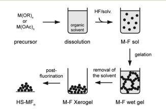
**Scheme 2** Illustration of the fluorolytic sol-gel synthesis starting from a metal alkoxide or carboxylate.
