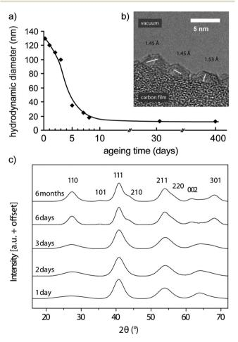
Fig. 12 Hydrodynamic diameter (a) and X-ray diffraction patterns (c) of the MgF<sub>2</sub> particles in the sol at different ageing stages, and HR-TEM image visualising MgF<sub>2</sub> primary particles from phosphonic acid stabilized sold (b). Reproduced from ref. 29b with permission of the Royal Society
