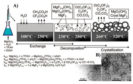
Fig. 1 (A) Scheme representing the deposition of porous MgF2 films on Si substrates by the TFA route; (B) TEM images showing the vesicle-like structures of the film prepared at 10 °C min<sup>-1</sup> under a dry atmosphere. Reprinted with permission from ref. 6a. © 2015 American Chemical Society.
