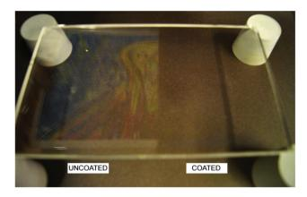
Fig. 19 Glass substrate coated by MgF<sub>2</sub> (right) whereas the left side is untreated. An image is shown above the glass and the mirror (left) or non-mirror (right) effect of each area while taking a picture from above can be seen.
