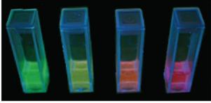
Fig. 16 Picture of transparent Eu<sup>3+</sup>- and Tb<sup>3+</sup>-doped CaF<sub>2</sub> sols (left) and the same sols excited with 366 nm (right). From left to right: CaF<sub>2</sub>:Tb10, mixture of 52% of CaF<sub>2</sub>:Tb10 + 48% of CaF<sub>2</sub>:Eu10, CaF<sub>2</sub>:Tb5.2,Eu4.8 and CaF<sub>2</sub>:Eu10; reproduced from ref. 44 with permission of The Royal Society of Chemistry.
