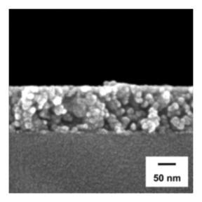
Fig. 20 Cross-sectional SEM image of  $MgF_2$  thin film annealed at 500 °C. Reproduced from ref. 33 with permission of The Royal Society of Chemistry.
