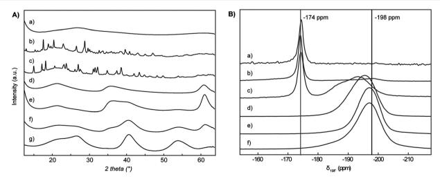
Fig. 11 (A) X-ray powder diffraction patterns of  $MgF_x(OCH_3)_{2-x}$  with x = 0 (a), 0.3 (b), 0.4 (c), 1 (d), 1.5 (e), 1.75 (f) and 2 (g), and (B) <sup>19</sup>F MAS NMR spectra of  $MgF_x(OCH_3)_{2-x}$  with x = 0.1 (a), 0.3 (b), 0.4 (c), 1 (d), 1.5 (e) and 1.75 (f); recorded in a 2.5 mm probe at 25 kHz. Reproduced from ref. 29b with permission of the Royal Society of Chemistry.
