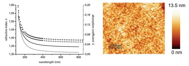
Fig. 18 Comparison of the refractive index n and absorption coefficient k of a MgF<sub>2</sub>-film prepared from a 0.15 M sol on a silicon wafer (solid lines) with values from literature (squares: e-pol and triangles: o-pol) for bulk MgF<sub>2</sub><sup>54</sup> between 150 nm and 800 nm (left). AFM image of a three step coated MgF<sub>2</sub>-layer on a silicon wafer calcined at 300 °C. Reproduced from ref. 53b (right) with permission of Elsevier.
