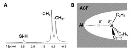
Fig. 14 (a)  $^1$ H MAS NMR spectrum showing the signals for surface-bound  $Et_3$ SiH ( $\nu_{rot} = 10$  kHz) with the SiH resonance at  $\delta = 3.45$  ppm. For  $Et_3$ SiH in  $C_6D_6$  solution, the resonance is observed at  $\delta$  = 3.85 ppm. (b) Schematic representation of ACF···H–SiEt<sub>3</sub>. Reproduced from ref. 26 with permission of the Royal Society of Chemistry.
