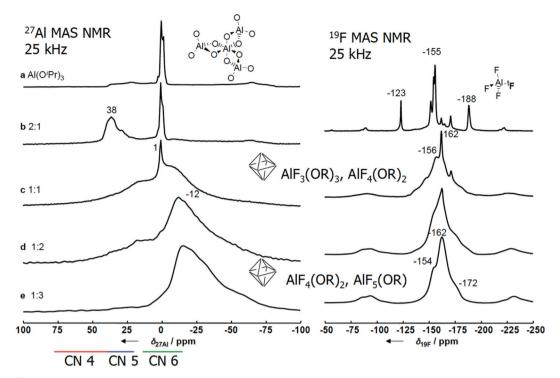
Fig. 5  $^{27}$ Al and  $^{19}$ F MAS NMR spectra of Al(OiPr)<sub>3</sub> and aluminium isopropoxide fluoride solids prepared with different molar ratios Al: F as given in the figure ( $\nu_{rot}$  = 25 kHz,  $B_0$  = 9.4 T). Reproduced from ref. 13b with permission of Wiley.
