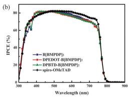
Fig. 3 (a) Photocurrent-voltage (J-V) curves of the solar cells with  $B[BMPDP]_2$  ( $\blacksquare$ ),  $DPEDOT-B[BMPDP]_2$  ( $\blacksquare$ ),  $DPBTD-B[BMPDP]_2$  ( $\blacktriangle$ ) and spiro-OMeTAD (♦) as the HTMs, respectively. (b) Corresponding IPCE spectra.
