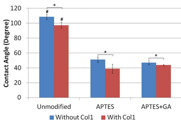
**Fig. 2** Average contact angles measured on unmodified and chemically modified PDMS surfaces, with and without Col1 coating. The data are shown as the mean  $\pm$  SD. \* $p$  value of  $<0.05$  between two groups under comparison. # $p$  value of  $<0.05$ , as compared to the modified PDMS surfaces with or without Col1 coating.
