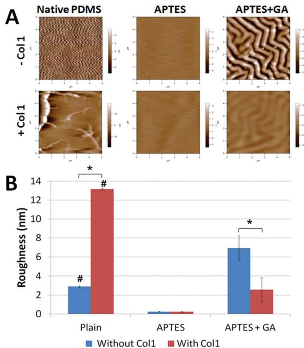
**Fig. 3** Substratum topography (A) and RMS roughness (B) of unmodified and chemically modified PDMS surfaces, with and without Col1 coating. \* $p$  value  $<0.05$  between two groups under comparison. # $p$  value  $<0.05$ , as compared to the chemically modified PDMS surfaces, with or without Col1 coating.
