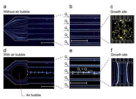
Fig. 5 Fluorescent flow tracer analysis: (a–c) normal cultivation conditions with equal flow rates inside all supply channels; (c) diffusive mass transport conditions inside the cultivation chambers; (d) air bubble is deployed at the fivefold channel junction resulting in (e) a temporary inhomogeneous laminar flow profile and different volume flows  $\Phi_1$ ,  $\Phi_2$ ,  $\Phi_3$ ,  $\Phi_4$  and  $\Phi_5$  and thus (f) laminar flow through the cultivation chambers (scale bar 25  $\mu$ m).
