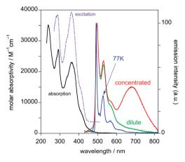
Fig. 2 Absorption and excitation ( $\lambda_{em} = 530 \text{ nm}$ ) spectra of PtL<sup>1</sup>Cl in CH<sub>2</sub>Cl<sub>2</sub> at 298 K (solid black and dashed purple lines); emission spectra under the same conditions for solutions of concentration  $1.8 \times 10^{-5}$  M (green line) and  $3.2 \times 10^{-4}$  M (red line) and emission spectrum at 77 K in diethyl ether-isopentane-ethanol (2:2:1 v/v) (blue line).
