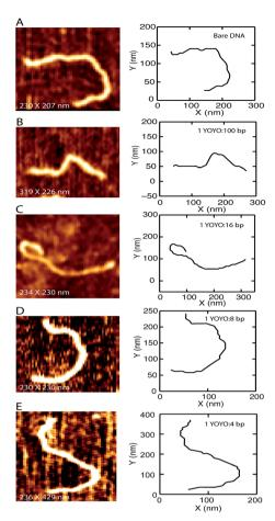
Fig. 2 Representative AFM images (left panel) of 1000 base pairs DNA molecules and their contours (right panel) when incubated with different ratios of YOYO to base pairs. (A) Bare DNA (B) 1YOYO per 100 base pairs (C) 1 YOYO per 16 base pairs (D) 1 YOYO per 8 base pairs (E) 1 YOYO per 4 base pairs.
