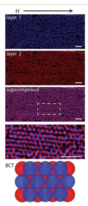
Fig. 8 Micrographs of adjacent layers in crystals assembled with pulsed magnetic fields. The superimposed image shows two layers depicted stacked in a way that suggests the structure of the crystal is body-centered-tetragonal (BCT) with the (110) plane coincident with the focal plane. The higher magnification image is indicated by the rectangular region in the superimposed image. The magnetic field is aligned horizontally across the micrographs. The scale bars are 10  $\mu m$ .
