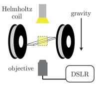
Fig. 1 A depiction of the experimental apparatus consisting of a Helmholtz coil spaced to receive a standard microscope slide suspended above the objective of an inverted microscope and imaged *via* a DSLR camera in a transmission geometry. Gravity acts normal to the slide and the magnetic field generated by the coils but parallel to the imaging path.
