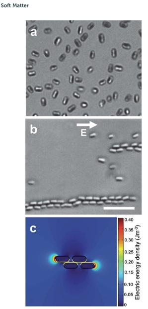
Fig. 3 Bright-field microscopy images of (a) side-coated Janus rods in absence of an electric field and (b) staggered chains composed of side-coated Janus rods assembled parallel to the electric field direction at 15 V mm $^{-1}$ , 100 kHz. The scale bar is 10  $\mu m$ . (c) Finite element modeling of electric energy density (Jm $^{-3}$ ) distribution around overlapping staggered side-coated Janus chain at 15 V mm $^{-1}$ , 100 kHz.
