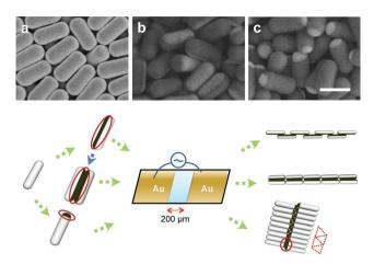
Fig. 1 SEM images of (a) homogeneous silica rods (L/D=2.1), (b) side-coated Janus rods, and (c) tip-coated Janus rods (or matchsticks). The scale bar is 2  $\mu$ m. (d) Schematic illustration of potential pathways for assembling these patchy particles into chain-like structures in an AC electric field.
