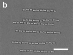
Fig. 2 Bright-field microscopy images of homogeneous silica rods in an applied electric field strength of 50 V mm $^{-1}$  at (a) 100 kHz and (b) 30 MHz. The scale bar is 10  $\mu$ m.
