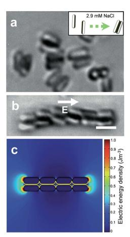
Fig. 4 (a) Janus rod doublets are formed by side-coated Janus rods with the addition of 2.9 mM NaCl. The inset shows the formation of Janus doublets from side-coated Janus rods. (b) A flexible doublet chain assembles parallel to the electric field direction at 20 V mm $^{-1}$ , 100 kHz. The scale bar is 3  $\mu m$ . (c) Finite element modeling of electric energy density (Jm $^{-3}$ ) distribution around a chain assembled from Janus doublets.
