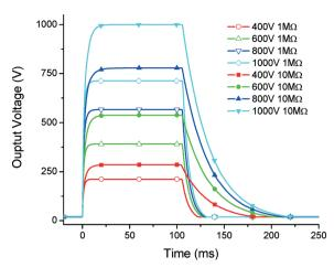
Fig. 13 High voltage power supply with 1000 V, 800 V, 600 V and 400 V setting with two different loading resistors, 10 M $\Omega$  and 1 M $\Omega$ . It shows the load influence on the output voltage as well as on the discharging time.
