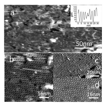
**Fig. 2** AFM and STM scans of a PTCDI-melamine network on HOPG in air. Images (a) and (b) are topographic AFM scans. Image (c) is a constant current STM image acquired at *I* = 5 pA and sample voltage 0.5 V. Image (d) shows adhesion distribution of the upper half of the area in (b). Inset on image (a) shows cross-section taken along the line shown in image (b).
