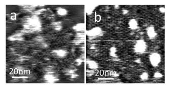
Fig. 4 AFM images of PTCDI-melamine network on  $MoS_2$  surface after (a) 1 minute and (b) 10 minute adsorption times.
