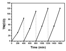
Fig. 3 Formation of CO in a 4-cycle repetition of irradiation at >420 nm for 400 min after CO<sub>2</sub> bubbling for 30 min in the dark; 10 mg Dye/S-TiO<sub>2</sub>/ **ReC** with 0.1  $\mu$ mol **ReC** and 1.5  $\mu$ mol Dye in the presence of 0.1 M SD and 10% (v/v) H<sub>2</sub>O.
