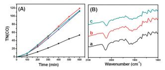
Fig. 2 (A) Plots of CO formation versus time in the absence  $(-\blacksquare -)$  and presence of 1.5 M 2,2,2-trifluoroethanol ( $-\bullet$ -), 3% (v/v) H<sub>2</sub>O ( $-\Delta$ -), and 10% (v/v) H<sub>2</sub>O (-▼-) for 10 mg **ReC** (0.1 μmol)/H-TiO<sub>2</sub>/Dye (1.5 μmol) in 3 mL DMF containing 0.1 M SD; irradiation at >420 nm. (B) IR spectra of ReC/H-TiO<sub>2</sub>/Dye in KBr discs (sample: KBr  $\approx 1:100$ ) before (a) and after irradiation for 100 min (b) and for 20 h (c).
