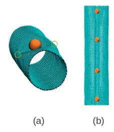
Fig. 4 (a) Transversal bucking caused by a large single point deformation. In this case  $I_p < L_t$  and the side rings indicate the location of the transversal stress focus points. (b) Uniform axial buckling and nanotube radial collapse induced by four equidistant localized deformations such that  $4l_p > L$
