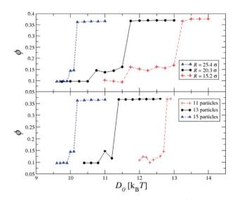
**Fig. 3** (Color online) Top panel: The onset value of collapse,  $D_0^*$ , increases as the nanotube radius R decreases because the nanoparticles need to deform against the larger curvature.  $K_b = 35 k_B T$  and N = 15 are kept constant. Bottom panel:  $D_0^*$  increases as the number of nanoparticles N decreases due to lesser collective deformation by the particles.  $K_b = 35 k_B T$  and  $R = 25.4 \sigma$  are kept constant.
