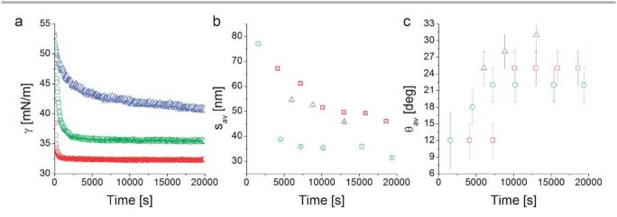
Fig. 4 Interfacial tension measurements from pendant drop tensiometry (a), fitted average inter-particle separation (b) and contact angle (c) from XR data modeling as a function of time for the nanoparticles L5 (□), L2.5 (○), and D2.5 (△).
