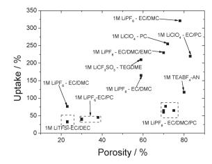
Fig. 3 Porosity vs. uptake for various electrolyte solutions incorporated into
