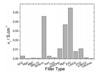
Fig. 4 Ionic conductivity for different filler types.
