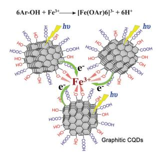
Fig. 7 Schematic illustration of the fluorescence quenching mechanism of the GCQDs in the presence of Fe<sup>3+</sup>. The top equation shows the formation of a complex between Fe3+ and 6 phenolic hydroxyl groups.
