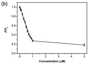
Fig. 5 (a) PL spectra of GCQD aqueous solutions with different Fe<sup>3+</sup> concentrations (from top to bottom: 0, 2, 50, 100, 200, 300, 400, 500, 600, 700, 800, 900 nM, 1 and 5  $\mu$ M, respectively). (b) The dependence of  $F/F_0$  on the concentration of Fe  $^{3+}$  ions within the range of 0–5  $\mu$ M. The excitation wavelength was fixed at 340 nm for all the PL spectra. F and  $F_0$  are the PL intensities at 445 nm in the presence and absence of Fe<sup>3+</sup> ions, respectively.
