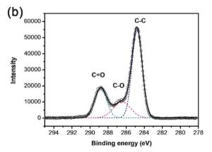
**Fig. 2** (a) Survey X-ray photoelectron spectrum of the GCQDs, only C and O signals are detected. (b) C 1s spectrum of the GCQDs. The C1s spectrum has been deconvoluted into three peaks at 284.6, 286.6 and 288.5 eV, corresponding to C–C, C–O and C=O, respectively.
