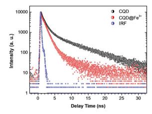
Fig. 8 Fluorescence decay traces of CQDs by TCSPC in the presence (red) and absence (black) of Fe<sup>3+</sup>. The blue line is the instrument response function.
