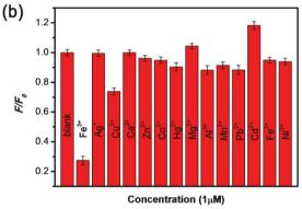
Fig. 6 (a) PL spectra of GCQD agueous solutions in the presence of different metal ions (the concentrations of the different metal ions are each 1 µM). (b) The different PL intensity ratios  $(F/F_0)$  of the GCQD solutions in the presence and absence of various metal ions.
