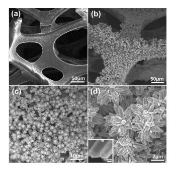
**Fig. 2** SEM images of the samples. (a) SEM image of 3D graphene foam. (b–d) SEM images of graphene/ZnO hybrids with different magnifications. The inset of (d) shows the morphology of a single ZnO nanorod at a high magnification.
