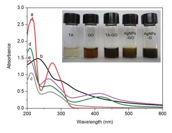
**Fig. 1** UV-vis absorption of aqueous dispersions of (a) TA; (b) GO; (c) TA-GO; (d) AgNPs–GO nanocomposites; (e) AgNPs–G nanocomposites. Inset: optical images of corresponding samples.
