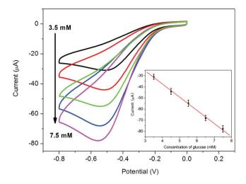
Fig. 6 Cyclic voltammograms of chitosan/GOD/AgNPs-G/GCE in O<sub>2</sub> saturated 1.5 mL real blood serum sample and 3.5 mL PBS solution (0.2 M, pH 7.4) in the presence of various concentrations of glucose: 3.5, 4.5, 5.5, 6.5 and 7.5 mM. Inset is the calibration curve (R = 0.998)corresponding to amperometric responses at the reduction peak (scan rate:  $50 \text{ mV s}^{-1}$ ).
