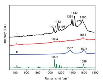
Fig. 3 (a) Raman spectrum of solid p-ATP, SERS spectra of p-ATP  $(1 \times 10^{-8} \text{ M})$  on (b) G, (c) AgNPs, and (d) AgNPs-G nanocomposites.
