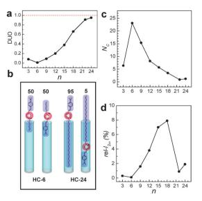
Fig. 6 The plots of DUO (a) and  $N_{\rm C}$  (b) versus n. A schematic illustration of the insertion of HC-6 into silicalite-1 channels with equal probabilities (50:50) for alkyl tail and head first and the contrasting behaviour of HC-24 which has a much higher probability (95%) to enter the silicalite-1 channels with the hydrophobic tail first than that for the head part first (c). The plot of rel- $I_{2\omega}$  versus n (d). (Adopted from ref. 47.)
