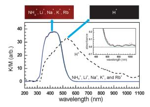
Fig. 13 Diffuse reflectance spectra of  $[2C^+, (PbS)_{OD}]_Y$  for  $C^+$ NH<sub>4</sub><sup>+</sup>, Li<sup>+</sup>, Na<sup>+</sup>, K<sup>+</sup>, Rb<sup>+</sup>, and H<sup>+</sup> (as indicated) after exposure to the moisture and the corresponding colors (maroon and black for C as indicated). (Adopted from ref. 80.)
