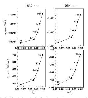
**Fig. 14** Plots of the  $\alpha_2$  (top) and  $n_2$  (bottom) values measured at 532 (left) and 1064 nm (right), respectively, with respect to the Sanderson's partial negative charge of oxygen  $(-\delta_0)$ . (Adopted from ref. 80.)
