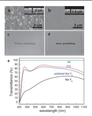
**Fig. 11** SEM images (top views) of zeolite-Y films grown on ITO glass plates before (a) and after (b) polishing and the corresponding photographs (c and d) and the corresponding transmittance spectra (as indicated) (e).
