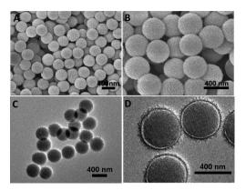
Fig. 2 (A, B) FESEM images and (C, D) TEM images of core-shell structured SiO<sub>2</sub>@nickel silicate nanospheres.
