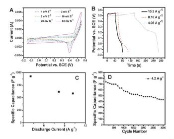
Fig. 4 (A) CV curves of NiS hollow spheres in the range of -0.15 V-0.55 V at various scan rates; (B) galvanostatic charge-discharge curves and (C) average specific capacitance of NiS hollow spheres at various current rates; (D) cycling performance of NiS hollow spheres at a current rate of  $4.2 \text{ A g}^{-1}$ .
