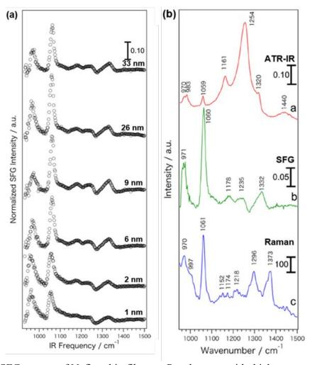
**Figure 8**. (a) SFG spectra of Nafion thin films on Pt substrates with thicknesses of 1, 2, 6, 9, 26, and 33 nm. (b) ATR-IR, VSFG, and Raman spectra of Nafion thin film with 33 nm thickness. Reproduced from ref. 95 with permission from [American Chemical Society], copyright [2014].
