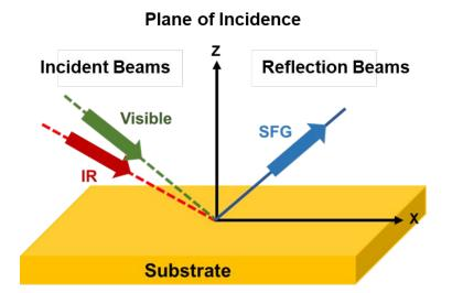
**Figure 2.** Illustration of two laser beams, a visible beam (green arrow) and an infrared beam (red arrow), incident on a substrate from which the sum frequency generation (SFG) laser beam is generated. The illustration is not to scale, and the area covered by the laser beams is on the order of one millimeter.
