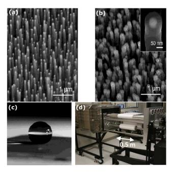
**Fig 11.** SEM images of (a) as as-grown carbon nanotube forest, (b) a carbon nanotube forest conformally coated by a 50 nm thick PTFE layer deposited by iCVD, and (c) a spherical water droplet on the PTFE-coated carbon nanotube forest. <sup>169</sup> (d) Schematic of a roll-to-roll iCVD system for the hydrophobization of large scale substrates. Figures are reproduced from <sup>169</sup> with permission from ACS.
