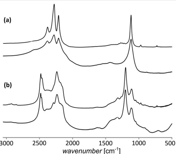
Figure 3. The FTIR spectra of the product of reaction between  $\text{K}[\text{Al}\{\text{OC}(\text{CF}_3)_3\}_4]$  and  $[n\text{Bu}_4\text{N}][\text{Y}(\text{BH}_4)_4]$ : (a) in dichloromethane with *ca.* 2.5 vol% of  $\text{CH}_3\text{CN}$  (upper curve) as compared to the spectrum of  $\text{KBH}_4$  (lower curve), (b) in pure dichloromethane (upper curve), as compared to the spectrum of  $\text{K}[\text{Y}(\text{BH}_4)_4]$  prepared mechanochemically.<sup>35</sup>
