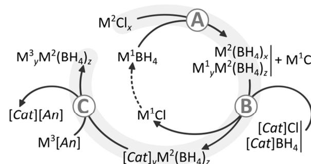
Figure 1. Synthesis of mixed-metal borohydrides, M<sup>3</sup><sub>y</sub>[M<sup>2</sup>(BH<sub>4</sub>)<sub>z</sub>], z = x + y. Steps A and B – synthesis and purification of borohydride precursor, step C – solvent-mediated metathesis. For Li[Sc(BH<sub>4</sub>)<sub>4</sub>] prepared this way: M<sup>1</sup> = Li, M<sup>2</sup> = Sc, M<sup>3</sup> = Li, [Cat] = [nBu<sub>4</sub>N], [Ph<sub>4</sub>P], [An] = [Al{OC(CF<sub>3</sub>)<sub>3</sub>}]<sub>4</sub>. Reproduced with permission from Ref.6.
