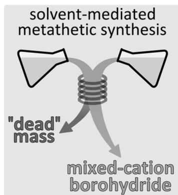
Figure 2. Schematic illustration of the combined key stages B and C (cf. Fig.1) of the synthetic protocol which enable separation of the "dead mass" (LiCl and the like) from the target product (complex borohydride). Reproduced with permission from Ref.6.
