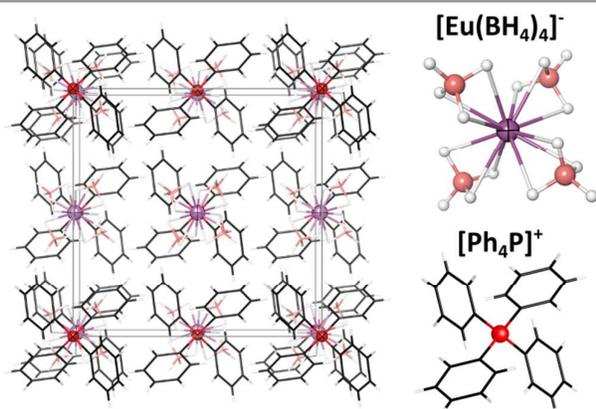
Figure 4. Unit cell of  $[\text{Ph}_4\text{P}][\text{Eu}(\text{BH}_4)_4]$ , presented here along the  $c$  axis, is composed of  $[\text{Eu}(\text{BH}_4)_4]^-$  and  $[\text{Ph}_4\text{P}]^+$  moieties which are drawn at the right side. Color code: black for C, white for H, pink for B, red for P, violet for Eu.
