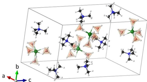
Figure 5. Unit cell of  $[\text{Me}_4\text{N}]_2[\text{Mg}(\text{BH}_4)_4]$ . Color code: black for C, white for H, pink for B, blue for N, green for Mg.
