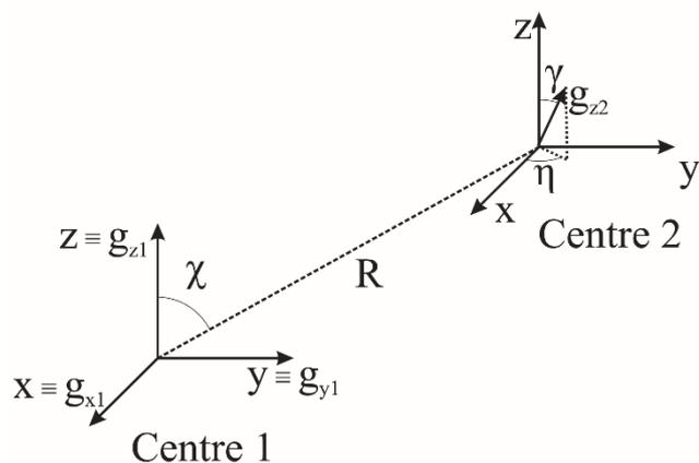
**Figure 5** Coordinate system appropriate to define relative position and orientation of two paramagnetic centres with axial symmetry. Polar angle  $\chi$  defines position, and Euler angles  $(\gamma, \eta)$  define orientation. Note that in an axial symmetry system  $\mathbf{g}_z$  is usually denoted as  $\mathbf{g}_\parallel$  and  $\mathbf{g}_x = \mathbf{g}_\perp$  as  $\mathbf{g}_\perp$ .
