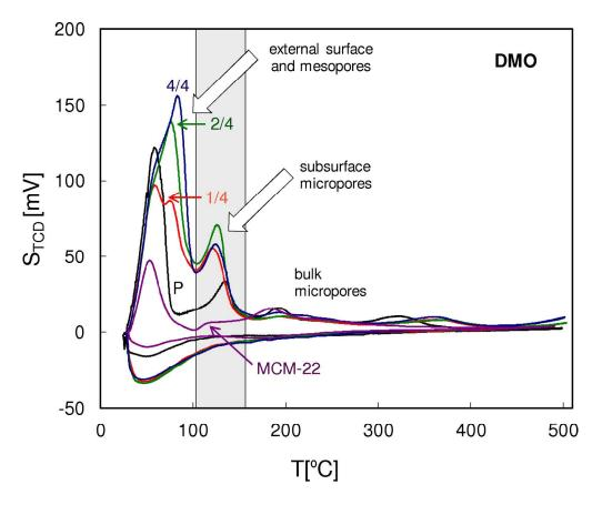
Fig. 13. QE-TPDA profiles of 2,2-dimethyloctane measured for the studied MCM-56 and MCM-22 zeolites at  $10^{\circ}$ C/min.
