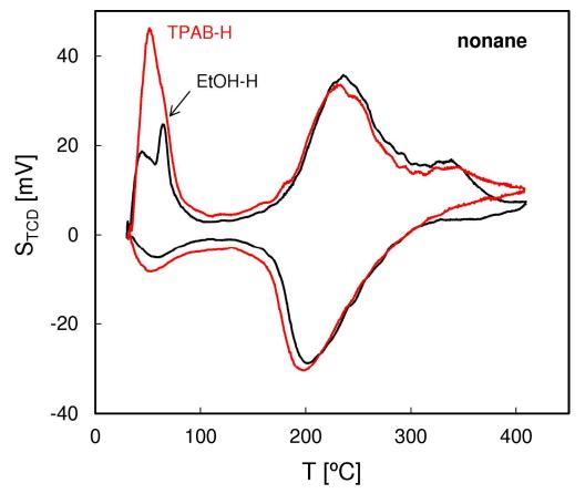
Fig. 5. QE-TPDA profiles of nonane measured for the studied ZSM-5 zeolites at 10°C/min
