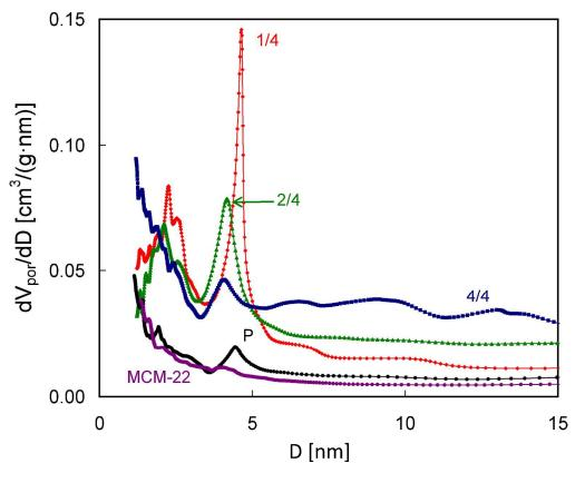
Fig. 12. Pore size distributions calculated from the desorption parts of the QE-TPDA profiles of nonane measured at  $2^{\circ}$ C/min
