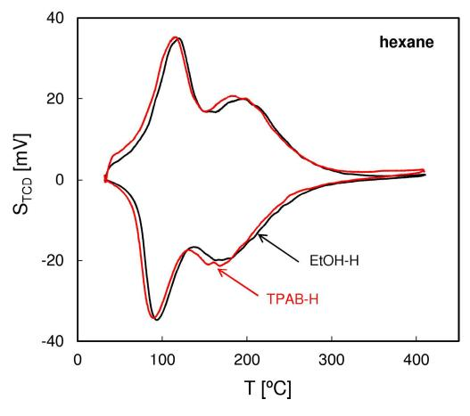
Fig. 4. QE-TPDA profiles of hexane measured for the studied ZSM-5 zeolites at 10°C/min
