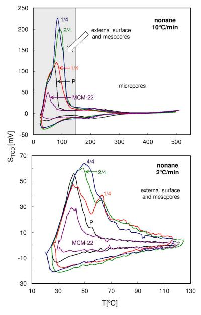
Fig. 11. QE-TPDA profiles of nonane measured for the studied zeolites MCM-56 and MCM-22 at 10 and  $2^{\rm o}\text{C/min}$
