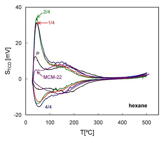
Fig. 10. QE-TPDA profiles of hexane measured for the studied zeolites MCM-56 and MCM-22 at 10°C/min
