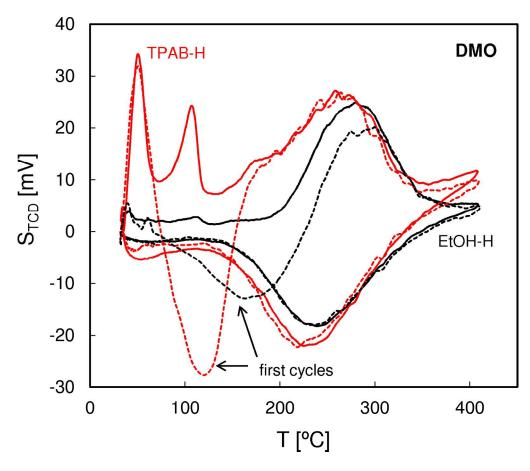
Fig. 6. QE-TPDA profiles of 2,2-dimethyloctane measured for the studied ZSM-5 zeolites at 10°C/min.
