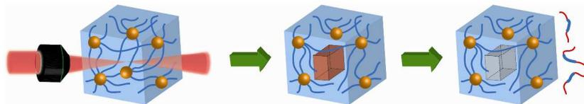
Light-induced disintegration of physically crosslinked hydrogel networks has been demonstrated by selective photodeprotection of self-assembled triblock copolymers. Physical crosslinks can be disrupted through light-induced uncaging of coumarin-based blocks using single- and two-photon absorption mechanisms. Photodegradable hydrogels exhibit promising applications as biomedical materials that can be manipulated using light at tissue-transparent wavelengths.
