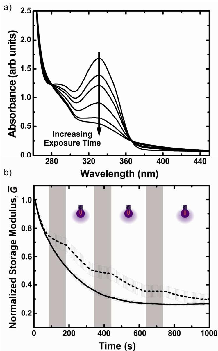
**Figure 2.** a) UV-vis spectra of poly(MAA-co-BHCMM)-PEG-poly(MAA-co-BHCMM) in DMSO solution before and after UV exposure. Uncaging is evident by the decrease of absorbance peak at 330 nm. b) The temporal evolution of normalized storage modulus  $\bar{G}$  is plotted for continuous (solid line) and intermittent (dashed line) exposure to UV irradiation. White (grey) vertical bars correspond to the presence (absence) of UV illumination.
