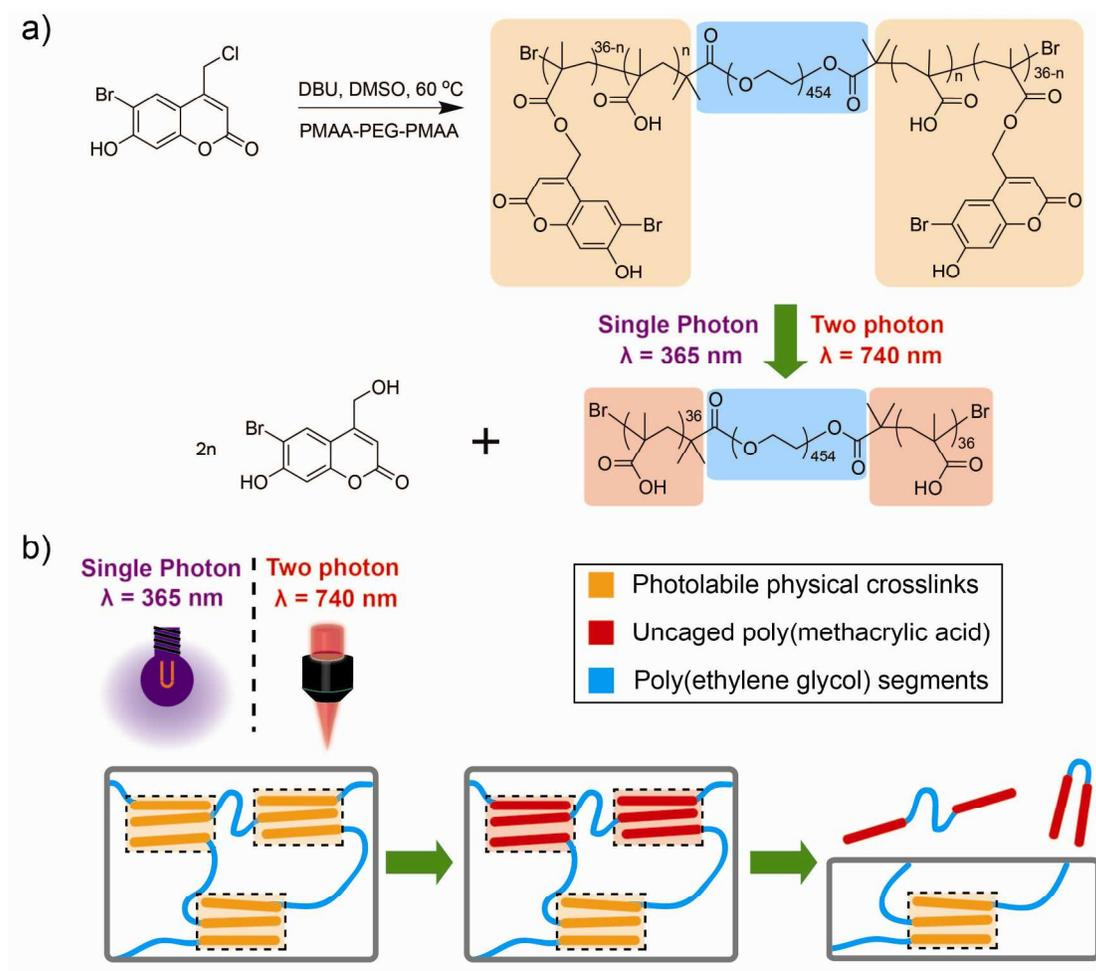
**Figure 1.** a) Synthesis and photodeprotection schemes for poly(MAA-co-BHCMM)-PEG-poly(MAA-co-BHCMM) ABA triblock copolymers is shown. Light-induced uncaging of PBHCMM segments yields water soluble PMAA-PEG-PMAA ABA triblock copolymers. b) A schematic illustration that describes the proposed mechanism of light-induced phase inversion and disintegration of physically crosslinked hydrogels.
