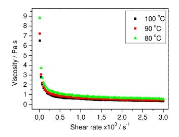
**Figure 4.** Viscosity *vs.* shear rate for  $[C_{16}C_{16}IM][BF_4]$  in the liquid crystalline temperature range (80 – 100 °C).
