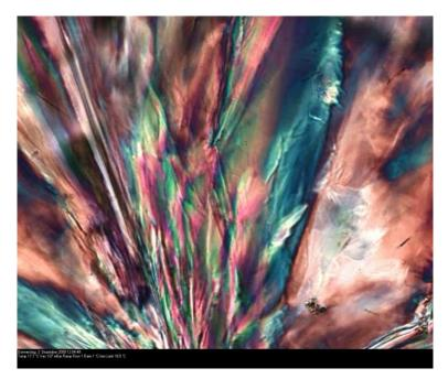
**Figure 3.** POM image of  $[C_{10}C_{10}IM][BF_4]$  at 17.7 °C (200× magnification). Liquid crystalline phase re-establishes after several minutes when cooling to 17.7 °C.
