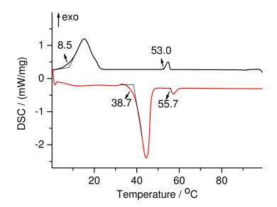
**Figure 6.** DSC of a mixed  $[C_{10}C_{10}IM][BF_4]$  and  $[C_{12}C_{12}IM][BF_4]$  in a molar ratio of 1:3.  $2^{nd}$  heating cycle (bottom),  $2^{nd}$  cooling cycle (top).
