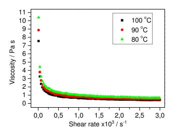
**Figure 5.** Viscosity *vs.* shear rate for  $[C_{16}C_{16}IM][ClO_4]$  in the liquid crystalline temperature range (80 – 100 °C).
