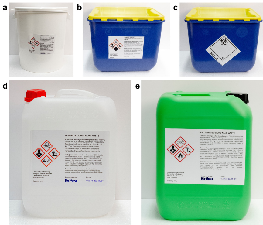
Fig. 3 Representative containers for nanowaste storage and transport. Adapted from Schwab et al. with permission from Springer Nature, Nature Nanotechnology , 18(4):317–321, copyright 2023. 14 a: White bin for solid nanowaste. b: Blue bin for solid biohazardous nanowaste. c: Example of dual storage/transport container with ADR 34 biohazard pictogram. The United Nations code 3291 stands for not otherwise specified clinical waste. d: White canister for aqueous nanowaste. e: Green container for nanomaterials in halogenated solvents. Contents must always be explicitly listed on the label. 35,36 Waste colors shown are examples and not legally binding. For more details on labeling, refer to the section ‘labels for storage and transport’ and the SI section ‘details on labeling nanowaste’.
