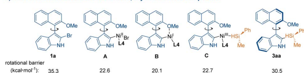
Scheme 2 Proposed reaction pathway and calculated rotational barriers.
