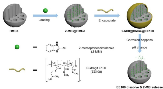
Fig. 4 Schematic illustration of the pH-responsive inhibitor system with Eudragit E100. Reproduced with permission 80 from Elsevier.
