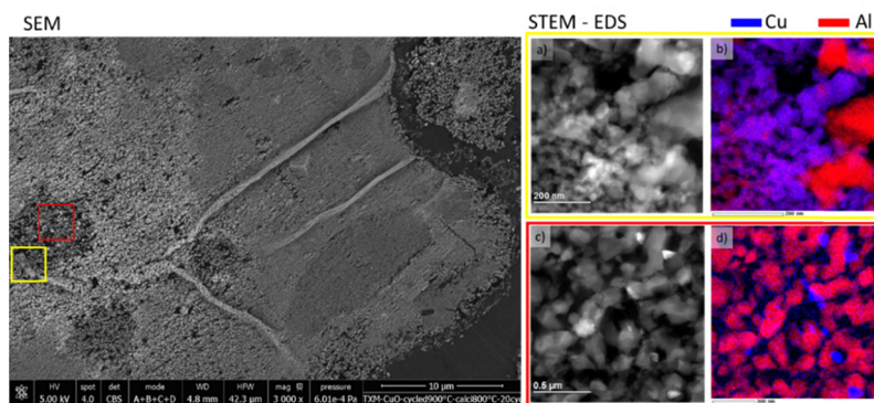
Fig. 8 (a), (c) STEM and (b), (d) EDS of 13 wt% \text{CuO}/\text{Al}_2\text{O}_3\text{-900} sample cycled 20 times at 900^\circ\text{C} carried out in TGA, displaying Cu-aluminate/ \alpha\text{-Al}_2\text{O}_3 phases.
