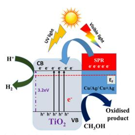
Fig. 9 A schematic illustration of the possible mechanism for SPRinduced electron transfer and co-catalytic activity during photocatalytic reaction of the Ag-Cu/TiO<sub>2</sub> nanocomposite
