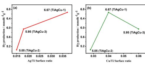
Fig. 8 (a) Variation of rate of hydrogen production with Aq/Ti surface ratio. (b) Variation of rate of hydrogen evolution with Cu/Ti surface ratio.
