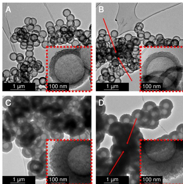
Fig. 4 Transmission electron micrographs of DC and SCD carbon spherogel samples after physical activation with CO<sub>2</sub>. (A) 35-nm-walled sample, SCD; (B) 35-nm-walled sample, DC; (C) 125-nm-walled sample, SCD; (D) 125-nm-walled sample, DC.
