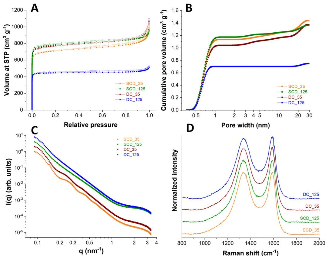
Fig. 5 Structural analysis of DC\_125; DC\_35, SCD\_125, SCD\_35. Nitrogen sorption isotherms (A) and pore size distribution curves (B) of directly carbonized (DC) and first supercritically dried and then carbonized (SCD) samples after physical activation with CO<sub>2</sub> at 900 °C for 90 min. (C) SAXS scattering curves; (D) Raman spectra of SCD and DC samples after CO<sub>2</sub> activation (samples are shifted vertically for better visibility).
