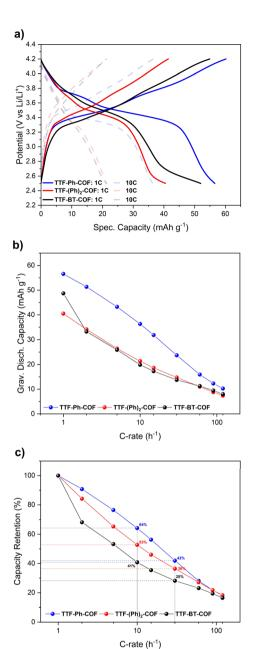
Fig. 6 Galvanostatic charge-discharge rate capability experiments of TTF-Ph-COF, TTF-(Ph)2-COF, and TTF-BT-COF, using a potential window of 2.5-4.2 V. (a) Galvanostatic profiles at different current rates. (b) Gravimetric specific capacity versus C-rate. (c) Capacity retention as a function of C-rate.
