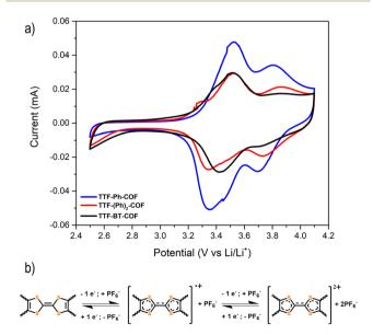
Fig. 5 (a) Cyclic voltammetry of TTF-Ph-COF, TTF-(Ph)2-COF, and TTF-BT-COF using 1 M LiPF<sub>6</sub> in EC/DMC (3/7 v/v) at a scan rate of  $0.5 \text{ mV s}^{-1}$ . (b) Redox mechanism of the p-type TTF moiety in TTF-COFs.
