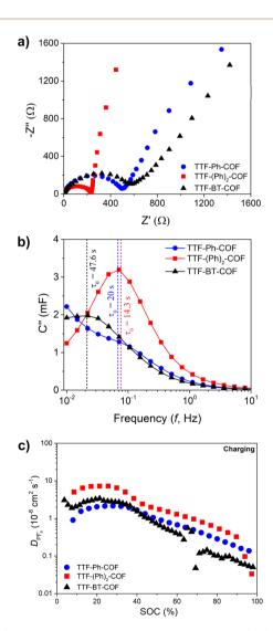
Fig. 7 (a) Electrochemical impedance spectroscopy (EIS) results at 3.7 V (vs. Li/Li<sup>+</sup>) upon charging, (b) imaginary capacitance analysis and characteristic time, and (c) diffusion coefficients of the PF<sub>6</sub><sup>-</sup> anion (charging) for TTF-Ph-COF (blue), TTF-(Ph)2-COF (red) and TTF-BT-COF (black).
