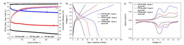
Fig. 8 Galvanostatic charge-discharge (GCD) long cycling experiments. (a) Cyclic stability and coulombic efficiency (square symbols) of TTF-Ph-COF, TTF-(Ph)<sub>2</sub>-COF, and TTF-BT-COF during long-term cycling at 2C, using a potential window of 2.5–4.2 V. (b) Galvanostatic profiles of the 2nd and 100th cycles. (c) Differential capacity analysis (dQ/dV) of the 2nd and 100th cycles.
